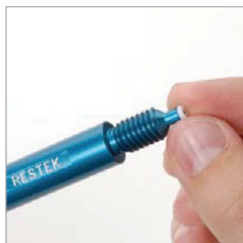
Place the O-ring over the tip of the tool.
