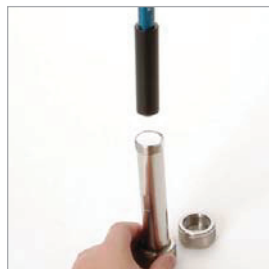
Place a filter at the top of the extraction cell.
