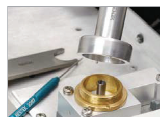
Easily loosen the nut by aligning the two pins on the bottom of the wrench with the two open slots on the nut...
