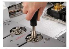
Simply slip the weldment removal tool over the weldment, then twist and remove the weldment. For speed and efficiency, the weldment stays secured in the weldment removal tool until you reattach it.
