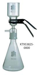
eliminates phthalate contamination that can occur when using silicone or neoprene stoppers. The support base has a coarseporosity glass frit and an integral vacuum connection, located above the drip tip to prevent contamination of the vacuum line with filtrate droplets. Each apparatus includes a funnel, an anodized aluminum clamp, a 47 mm fritted glass support base, and a filtration flask.
